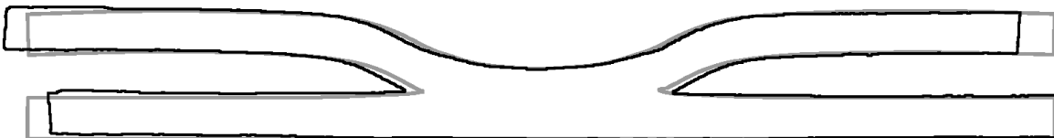
Fig.3: Comparison between the cross-sections of the numerical result with increased strain rate sensitivity (grey) and the experimental result (black).
