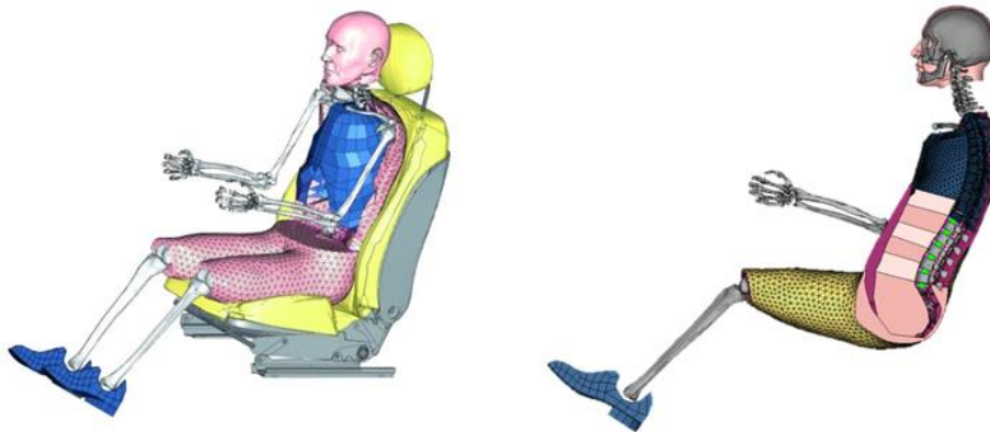
Fig.1: Wölfel Group's FE-human-body model CASIMIR with (left) and without (right) seat model.
