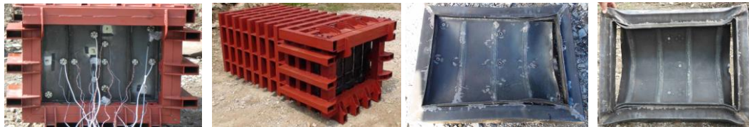
Reduced scale chamber model for internal blast test and damage configurations
