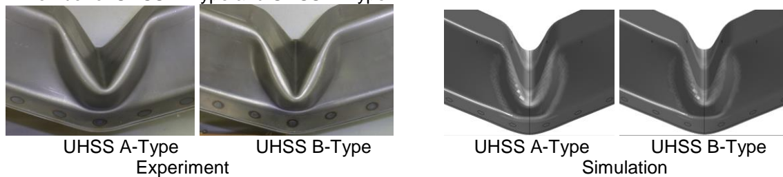
Fig.2: Comparison of numerical and experimental results for 3-point bending test of HAT member
