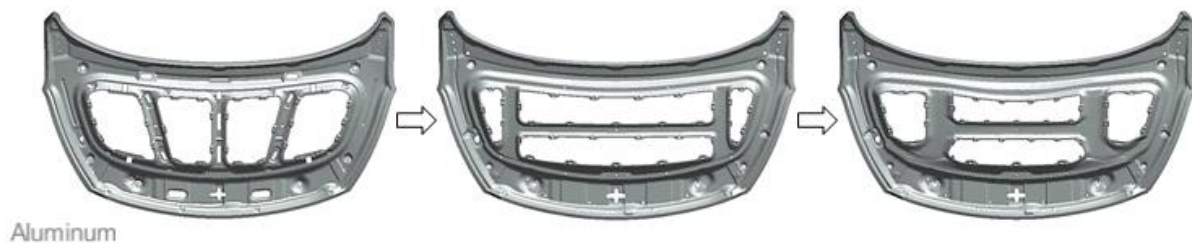
Fig.4: Initial design (left), design after topometry optimization (center) and design after shape optimization (right) of the inner aluminum panel.
