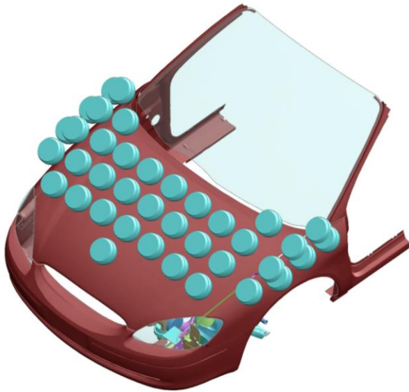
Fig.2: Multiple build of many LS-DYNA models based on target points.
