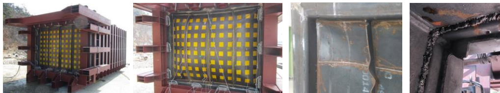
Partial chamber model for internal blast test and damage configurations
