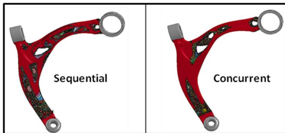
Fig.2: Resulting deformed structures of trade-off from running the sequential topology optimization of stiffness and energy absorption (left), and concurrent scaled weighting topology optimization, resulting from an equal preference of compliance and energy absorption (right).
